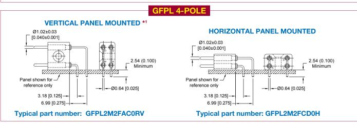
NOTE: \*1 When viewing the connector from the rear with the "A" contact position down, the panel on the left dictates "L" code while the panel on the right dictates "R" code. See ordering information page "Step 5".
