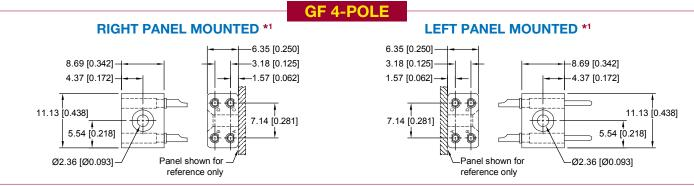
NOTE: \*1 When viewing the connector from the rear with the "A" contact position down, the panel on the left dictates "L" Code while the panel on the right dictates "R" code. See ordering information page "Step 5".
