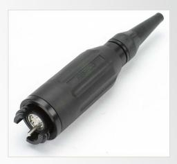
The connectors are terminated using an epoxy-polish ferrule termination process with standard fiber optic termination tools and equipment. The terminated ferrules are simply inserted into the expanded beam housing and fixed in place via a spring and cover-plate. Ferrule alignment to the lenses is achieved automatically by the unique optical arrangement developed and patented by Cinch-Fibreco.
