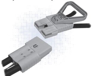
SBE® and SBX® connectors can integrate up to 8 auxiliary power / signal contacts along with the two primary power circuits. Sequencing within auxiliary positions is possible using the 4 pin lengths available in the 1x4 auxiliary connector. SBE® and SBX® offer touch safe housings.
